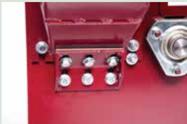
Easy to adjust anvil for maximum cutting performance.
